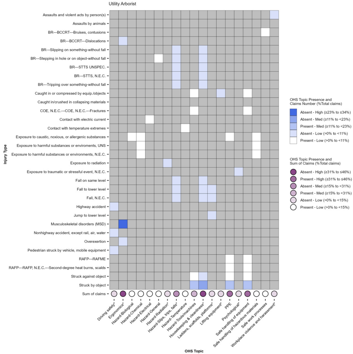
Figure 4.40.2: Heat map of the presence of each OHS topic and sum of claims of injury types linked to the OHS topic. Sum of claims in each trade is presented as a percentage of the total claims. The following OHS topics were identified in the apprenticeship standard but are not presented on the heatmap because we did not make a priori links to any injury type: communication, emergency preparedness, hazard-fire, and legislation. OHS topics that were not identified in the apprenticeship standard are denoted with an asterisk. See Appendix A for details on abbreviations.
