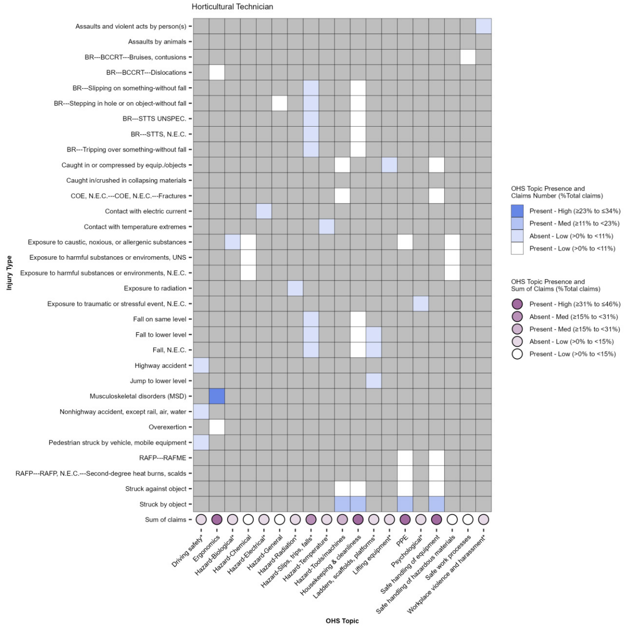
Figure 4.24.2: Heat map of the presence of each OHS topic and sum of claims of injury types linked to the OHS topic. Sum of claims in each trade is presented as a percentage of the total claims. The following OHS topics were identified in the apprenticeship standard but are not presented on the heatmap because we did not make a priori links to any injury type: communication, emergency preparedness, legislation, lockout/tag out, and psychosocial. OHS topics that were not identified in the apprenticeship standard are denoted with an asterisk. See Appendix A for details on abbreviations.
